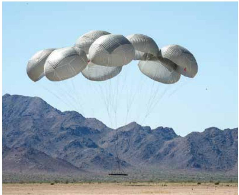
▲ **A 19,000 kilogram test** of a cluster of eight G-16 parachutes.
