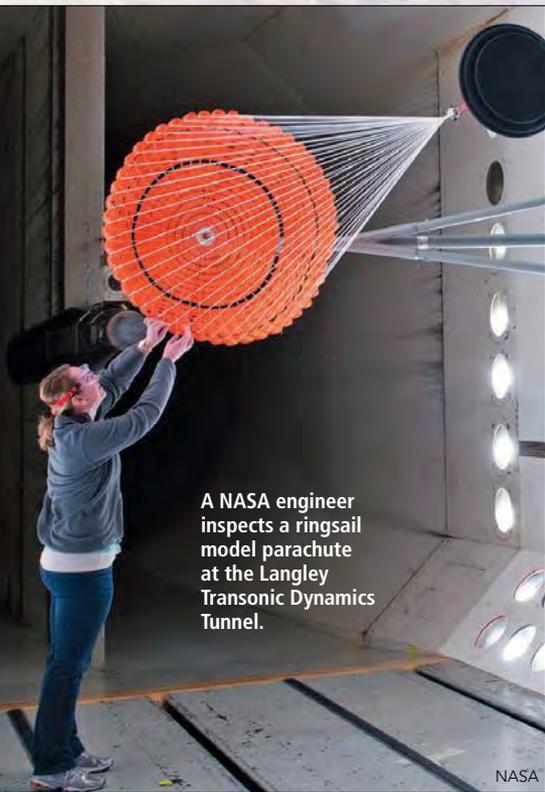
A NASA engineer inspects a ringsail model parachute at the Langley Transonic Dynamics Tunnel.
