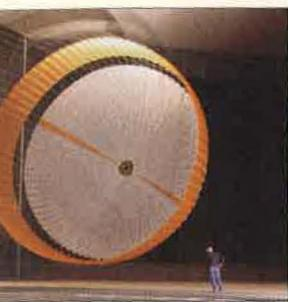
MSL parachute tests were conducted in the NASA Glenn Unitary wind tunnel.
