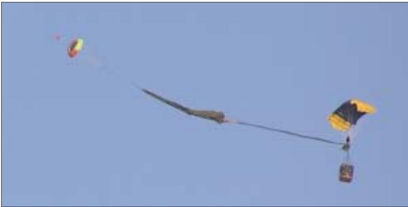
*The Screamer parafoil system deploys a secondary parachute for landing.*
