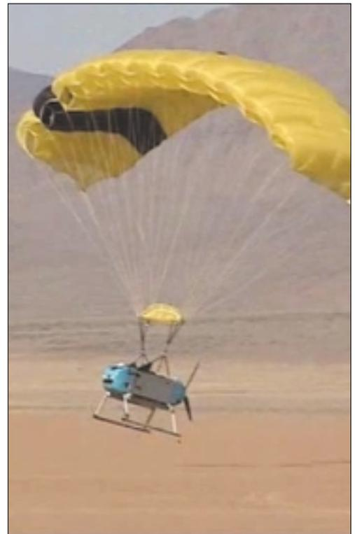
The Army powered parafoil system uses self-guided navigation to serve as an inexpensive unmanned aerial vehicle.
